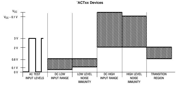
Figure 3-4b. Test Input Signal Levels
