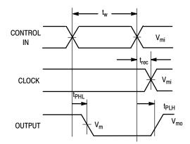
Figure 3-6. Propagational Delay, Pulse Width and t<sub>rec</sub> Waveforms
