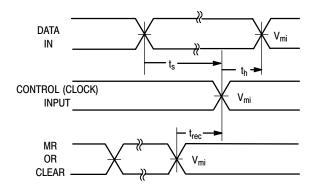
Figure 3-7. Setup Time, Hold Time and Recovery Time
