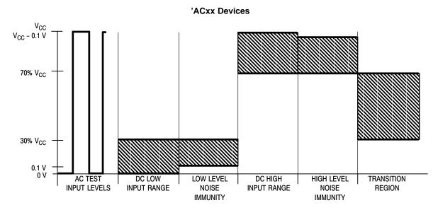
Figure 3-4a. Test Input Signal Levels
